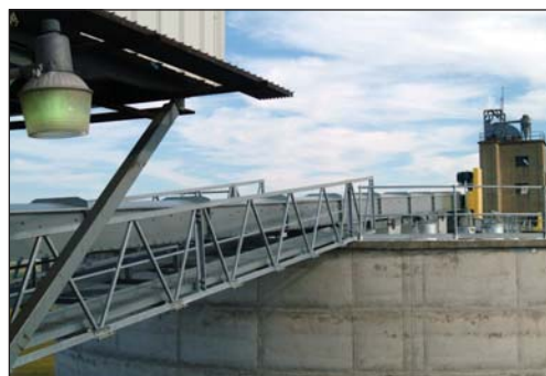
One of two 20,000-bph Union Iron Works drag conveyors leading out to the new tanks. Ground-level photos by Ed Zdrojewski.
