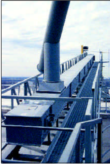
New 12,000-bph HSI drag conveyor carries grain out to the new west-end storage tank. Photo by Ed Zdrojewski.
